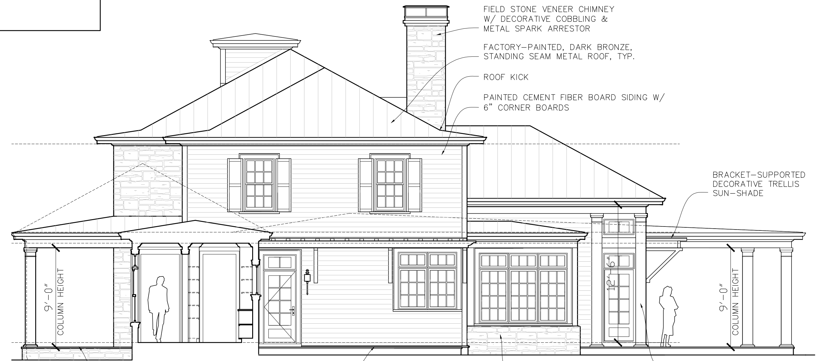
EAST ELEVATION/SECTION THROUGH HALL/PANTRY 3/16"=1'-0"
